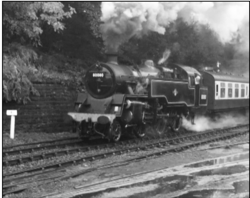
British Railways Standard 2-6-4T class 4MT No 80080 on the preserved East Lancashire Railway, Bury.
